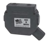
The PRINCE model RD-400 is a constant volume priority divider. It can be used in applications where two circuits are to be supplied by a single pump such as power steering systems. In operation the flow of oil supplied to the inlet is divided into two flows, the priority flow and the excess flow. The priority flow will remain nearly constant with variations in pressure on either the priority or excess flow port and will also remain nearly constant with variations in the inlet flow.
