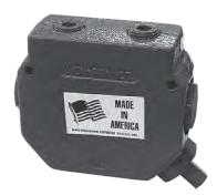
The PRINCE model RD-500 is an adjustable constant volume priority divider. This valve provides the same function as the PRINCE model RD-400 except the priority flow is adjustable from 2 GPM to 12 GPM. The priority flow is set using the adjusting screw and is then locked in place to maintain setting. This allows setting to be fine tuned in the field to the exact flow needed.
