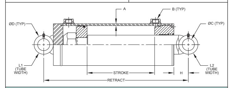
Rods are sized for a maximum safe push load (2:1 safety factor) given in the table. This is based on the pin configuration shown with no center support.
