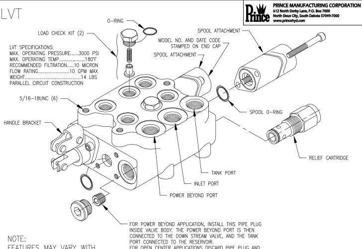
FEATURES MAY VARY WITH MODEL NO. CONSULT CATALOG PARTS MANUAL AVAILABLE AT www.princehyd.com FOR OPEN CENTER APPLICATIONS DISCARD PIPE PLUG AND PUT A STEEL PLUG IN POWER BEYOND PORT. FOR CLOSED CENTER APPLICATIONS, INSTALL PIPE PLUG AND PUT A STEEL PLUG IN THE POWER BEYOND PORT.
